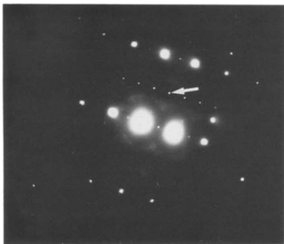
Figure 11 SADP from the same area as in Fig. 8, but with zone axis fcc [012].
