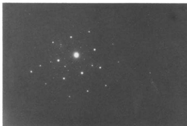
Figure 14 SADP of the M_{23}C_6 carbide particle and the surrounding matrix shown in Fig. 13. [001] Zone axis.
